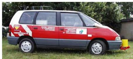
Fig. 1. : Vehicle for thermal mapping
